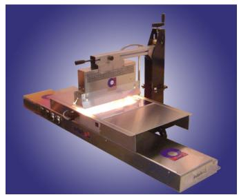
adphos PBTs (Platen Based Transports) are companion products for x-y inkjet plotters. PBTs allow for "production" drying, sintering and curing in a lab scale device. PBTs are available in two configurations with both stationary and motor driven platens. Both systems include vacuum plate (and air hold down) to maintain product integrity during processing.
