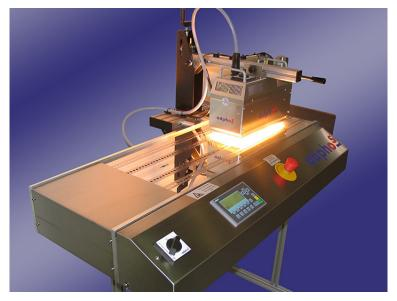
The adphos NIR-MiniLab is a flexible drying and curing system for research and development or prototype production of printed electronics or other printing applications with inks applied via flexographic, screen, gravure or inkjet printing.
