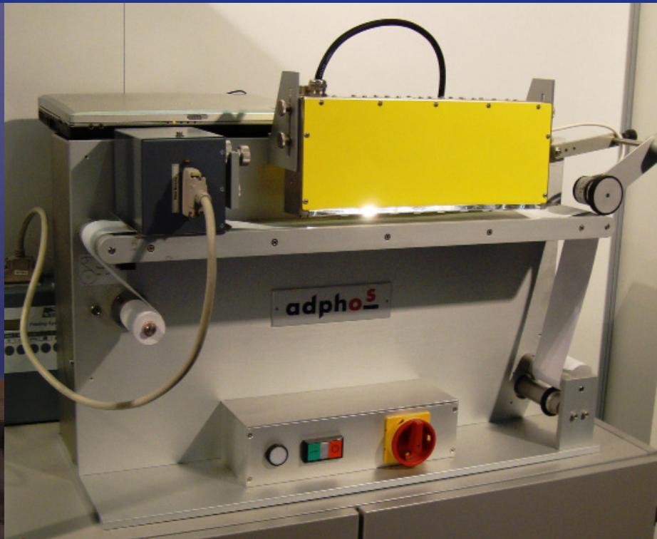
Adphos R2R (Roll-to-Roll) Transport Systems are a family of table top laboratory and pilot production transports for testing and validation of drying, curing and sintering applications for a multitude of inkjet technologies.
